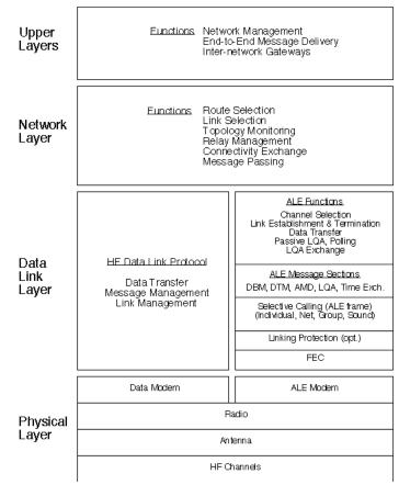
Figure 1: HF Automation Functions
