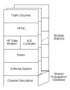
Figure 2: Simulator Structure
