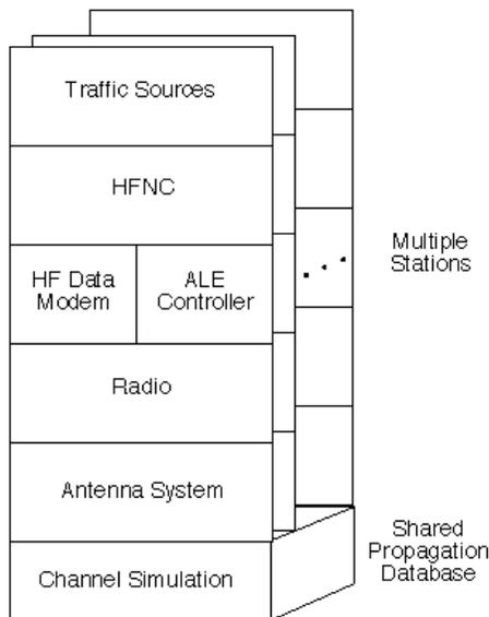
Figure 2: Simulator Structure
