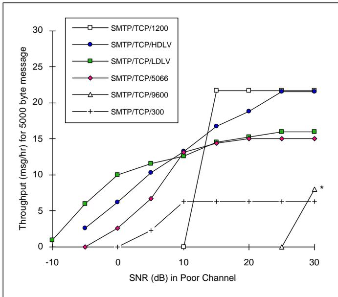
\* The throughput for 9600 bps at 30 dB reflects an artificial reduction of the TCP maximum timeout to 30 seconds. Without this modification, throughput was reduced to less than 1 msg/hr by the slow retransmission rate.
